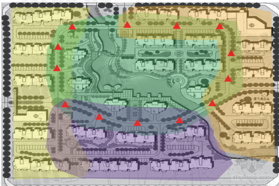
Fig7.1.1 Control Point setting for Data Stitching
